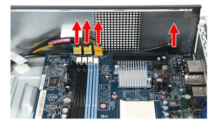
6. Remove the front I/O and card reader board bracket.
